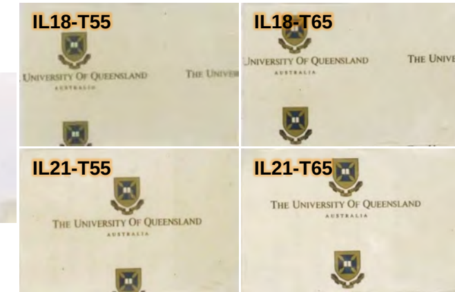
Starch films plasticised by water:[C 2 mim][OAc] prepared by hot-processing at 55–65 °C
